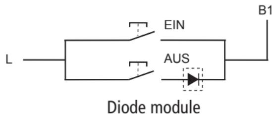
Push button ON: Switch on / dim up
