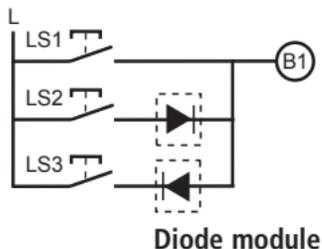
Light scene 1 can also be activated if buttons LS2 and LS3 are pressed simultaneously. This makes it possible to save using button LS1.
